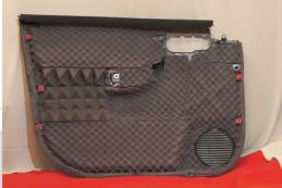
reduce distortion in mid-low frequencies. It is important to cover the inside of trim panels with SilentCoat Sound Absorber to reduce the penetrating noises as much as possible.
