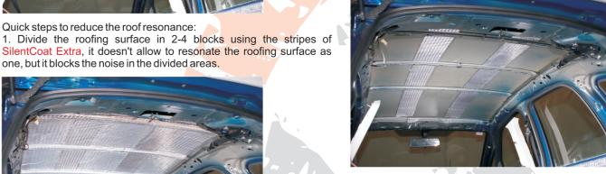
2. Cover the remaining big surfaces with SilentCoat. The application of SilentCoat doesn't increase the weight. Use SilentCoat Extra for more serious installs.
